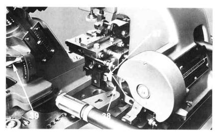
The mechanical action of the stop lever (28), the ratchet, the weight and the actuating lever itself is precisely the same as when casting leads and strip rules as already explained, except that the longer stroke of the actuating lever which results in the blade stop being withdrawn does not in this case operate the cutter cams.
