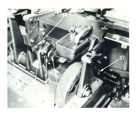
10.4 Type carrier cam lever plunger
