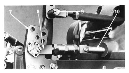
b) The intermediate lead clamp lever (14); a complex lever and rod, which connects to the lead clamp lever (13) located on the mould, its function being to clamp the cast strip in the mould and hold it firmly in position whilst the next fusing cast is being made immediately behind it.
