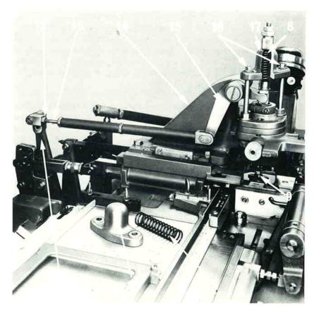
The matrix lifter stop collar must now be released and carefully adjusted so that the paper is just (and only just) free to move between the mould and the matrix. You must then lock the stop nut (5) and check the setting again (this time, checking with three thicknesses of paper, which should just hold) adjusting accordingly if necessary until it is correct.
