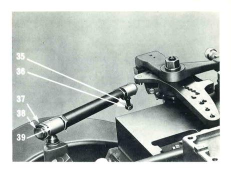
e) The mould blade slide drive lever connecting tube (5); which transfers the mould blade cam lever movement to the intermediate lever.
