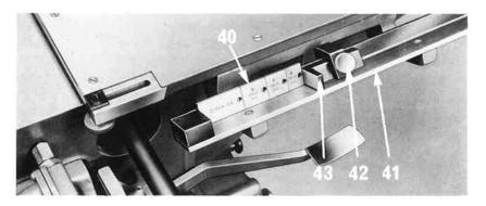
These measure gauges (40) are used in the length gauge (41) which is mounted just off the left-hand edge of the galley, adjoining the matrix box tray (45). They are used in the required combination to produce the desired measure (up to a maximum of 60 ems), the sliding jaw (43) being moved into position against the gauges (which must be an exact 'sliding' fit) and locked with the knurled clamp screw (42); the strip then being checked and measured in the gauge as illustrated.
