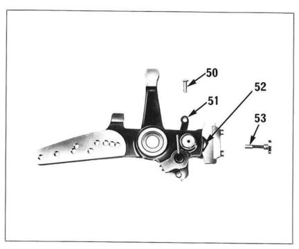
9.14 Replacing the plunger spring
