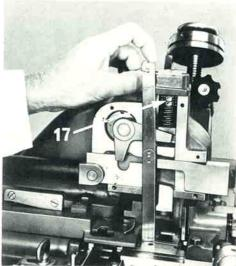
This adjustment causes the matrix lifter lever to be brought into operation by the traverse of the matrix lifter lever lock wedge, much earlier than is the case when casting type; and it similarly gives a greater degree of movement to matrix lever, thereby raising both the lifter (12) and the core the required distance to permit the product to be ejected from the mould.
