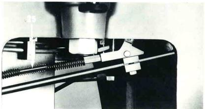
produce the continuous strip. The matrix lifter attachment connects with the matrix cam lever (27), via the upper of the two cam lever holes. It is fitted to the counter bracket as required, being passed through the aperture in the bracket to the rear of the lead clamp intermediate lever spring box (26). The matrix lifter bracket (18) is secured to the counter bracket (3) by the  $\frac{1}{2}$ in hexagon screw (17).
