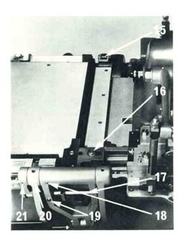
14.9 Removing the cutter actuating lever
